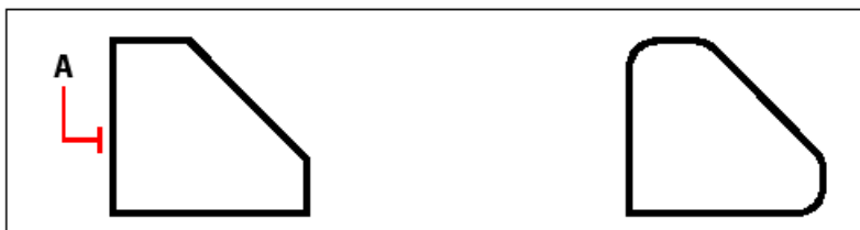
Select a polyline (A) – Result after filleting
