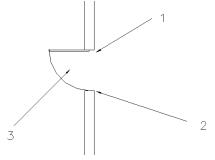
this value. Finally, the third point is inserted freely either on the one side of the wall or the other, since you simply determine the half-plane side towards which the door is placed.
