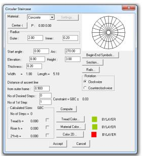
Regardless of the specific type, once the definition points and height are determined. click the you can Calculations button to view the results the various calculated staircase parameters, such as the step and the vertical stair surface, the number of stairs etc. In the lower left part of the window, there are some useful indications (b, h and 2h+b) showing the good compliance of the stair (boxes ticked).
