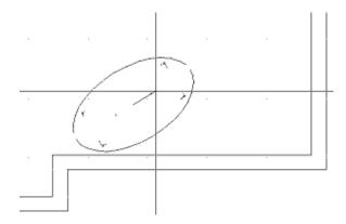
Left click to finalise the placement of the object. Note that, once the indication "scale xy" (on the top left) is activated, you can zoom in (or out) the corresponding symbol by x and y during the symbol placement. This is done by moving the mouse, immediately after you have placed the selected symbol on the drawing. The user can easily comprehend the way symbols are placed on ground plans running various relative tests.
