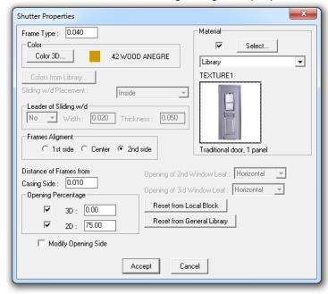
Finally, the **Modify opening side** option serves to define the direction of the opening side in case you want to change the default value. The **Reset from local Block** and **Reset from General Library** serve to modify the properties of the shutters that you have introduced within your drawings. Among the shutters and openings attributes, the user can define window-sills, cornices, labels and many other items.
