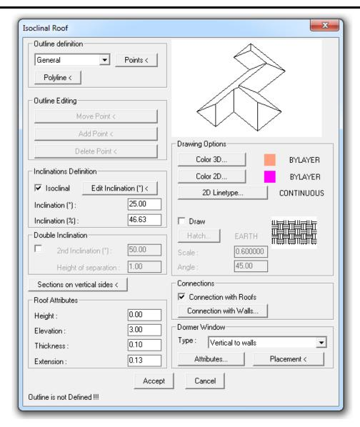
To define this type of roof, select **Points** and determine all the edges on the ground plan one by one (right click after determining the last point) or select **Polyline** and point on a closed polyline (the outline of which must have been already drawn). In this dialog, you can also define the inclination, height, thickness, level and distance of the roof from the outer sides. More specifically, the data are the following:
