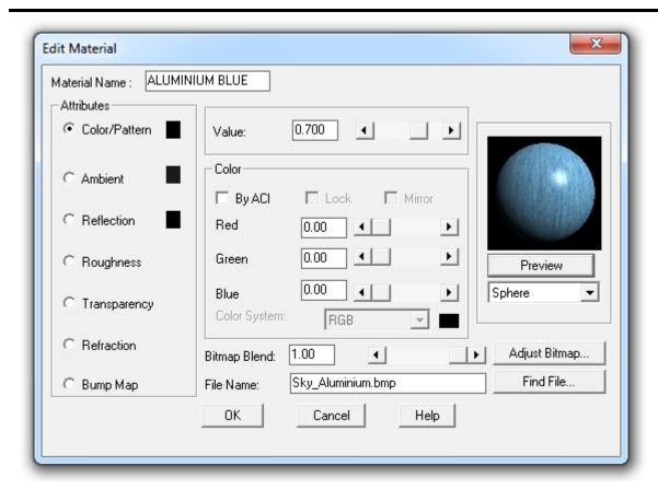
More specifically, you can modify each of the material **Attributes** that appear on the left side by specifying a **Value** with the sliding bar on the upper side. You can also modify **Color** by altering the mixtures of Red, Green and Blue or selecting between the RGB and HLS color systems. More specifically, the material properties which can be modified are **Color/Pattern**, **Ambient**, **Reflection**, **Roughness**, **Transparency**, **Refraction**, **Bump-Map** and **Adjust Bitmap**.
