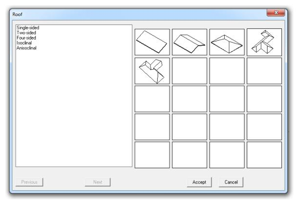
Depending on the selected roof type, a dialog box appears, prompting the user to enter the characteristic points of the roof, the roof height, the distance it protrudes from the wall etc. For example, selecting an Isoclinal roof displays the next dialog box.
