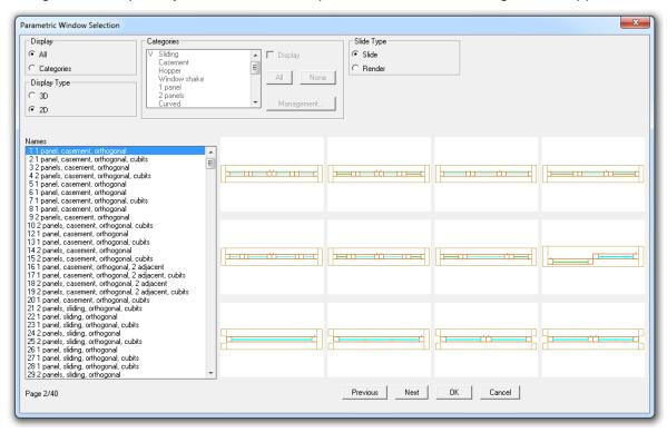
2. **User-defined Parametrical Window:** This option serves to select a window type that has been drawn freely by the user. The whole procedure for drawing new windows from scratch is described in the User's Guide.
