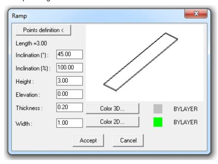
The program can also create **Free-Route Ramps** which are defined in a similar way to the free-route staircases, that is using a polyline that corresponds to the ascension line and the outlines that determine the boundaries of the ramp.
