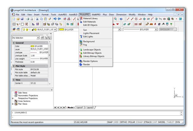
All these commands can be selected from the menu or from the **Render** toolbar that looks like the figure below. If you cannot see this toolbar, run the **View -> Toolbars** command and activate the **Render** option in the window with the checkboxes. Then the toolbar appears on the screen (and it can be positioned wherever the user wishes).
