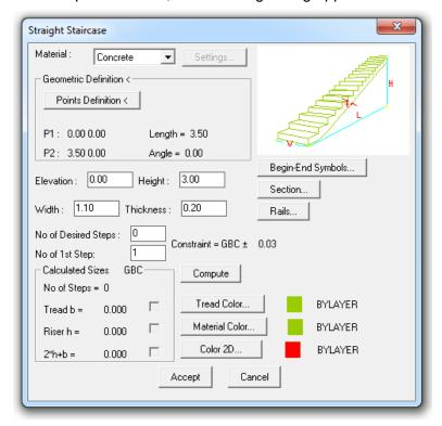
The determinant features of such a staircase are its "Definition Points", which have to be provided. When you click the **Point Definition** button, the programme prompts for the following characteristic points of the staircase:
