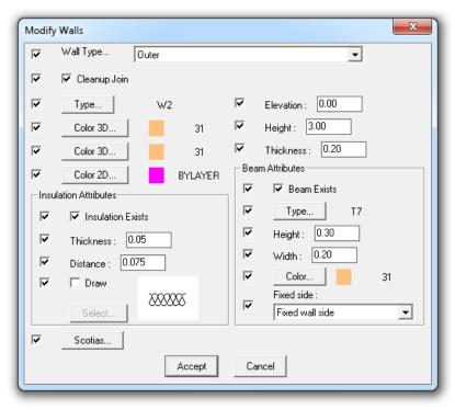
This command is also activated by successively selecting via left clicking the desired walls and then by right-clicking and selecting **Properties**.
