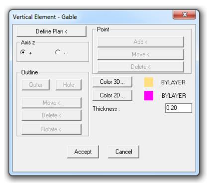
The **Plane Definition** option specifies on the ground plan the first and the second point of the axis relatively to which this element will be defined. Once these two points are specified, the programme automatically shows the view corresponding to the determined
