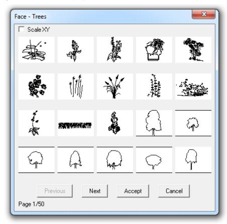
Placement is carried out through the known capabilities of progeCAD. More specifically, in the selected library symbol or drawing screen, press <Enter> on the symbol you desire and then press **OK**. During insertion, the program prompts only for the position where the drawing should be placed.
