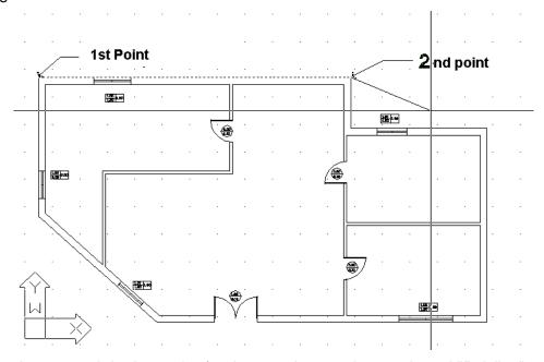
After having entered the last point (or, in case that you have selected "Polyline", after you have closed the polyline) you need to click the right button in order to view the "Roof" dialog box. Then, by clicking "OK" you see the isoclinal roof (with its ridges) being drawn:
